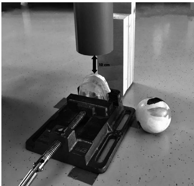
**FIGURE 1** Test setup. The polymethylmethacrylate (PMMA) dental model with mouthguard was placed into a clamp underneath the tube with the occlusal surface perpendicular to the ground with 10 cm distance to the tube
