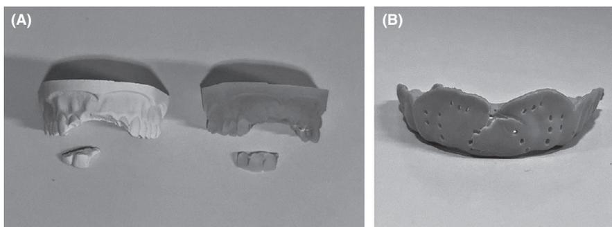
**FIGURE 3** A, Breaking pattern of a plaster and a polymethylmethacrylate (PMMA) dental model after impact. B, Damaged SISU mouthguard after impact
