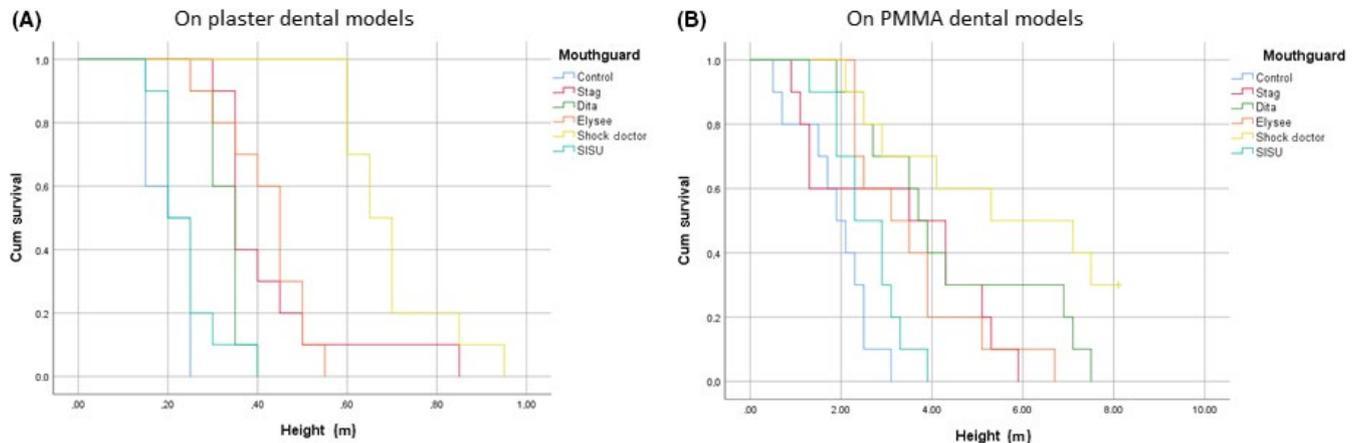
**FIGURE 2** Survival curve of different mouthguards and controls at different heights (in meters). A, on plaster models. B, on polymethylmethacrylate (PMMA) dental models, where 3 PMMA dental models with Shock Doctor mouthguard did not broke at maximum high of 8.10 m
