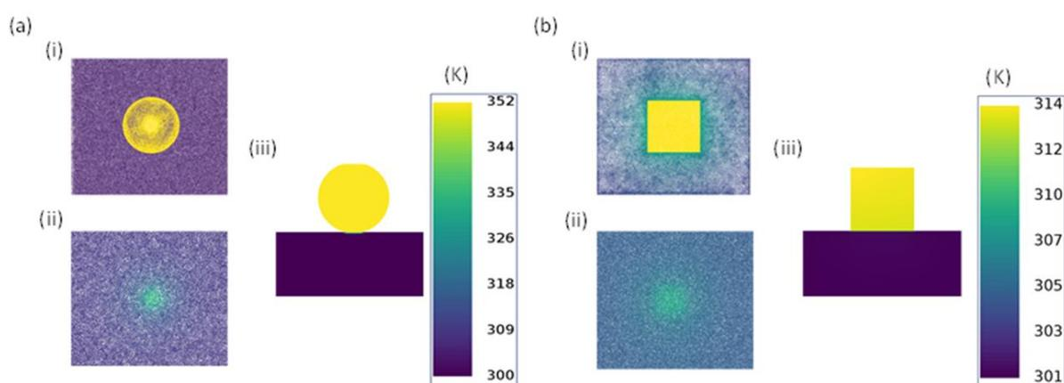
**Fig. S6: Local heating calculations on plasmonic nanoconstructs.** (a,b) Optically induced heating for NPoM and NCoM nanocavities. (i) Top surface, (ii) 3 nm below the substrate, and (iii) cross-section. Local heating of NPoM reaches 352 K compared to 314 K for NCoM. Ambient temperature is 300 K, irradiation is at 633 nm and optical intensity is 1 mW/ $\mu\text{m}^2$ .
