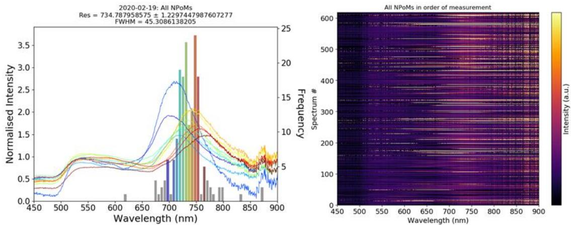
**Fig. S2: Dark-field spectra distribution of NPoM plasmonic constructs with MPA as a dielectric spacer.** All dark-field spectra are averages (lines) of all spectra and each histogram indicates the occurrence (left). Consecutive dark-field spectra of more than 600 nanoparticles on top of each other (right). Bright (dark) colours correspond high (low) scattering intensity.
