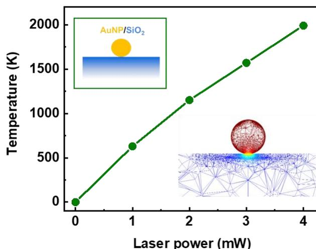
**Fig. S7: Heating of Au nanoparticle on SiO<sub>2</sub> substrate.** Optical heating of Au nanoparticle (80 nm) vs laser power at a wavelength of 633 nm.
