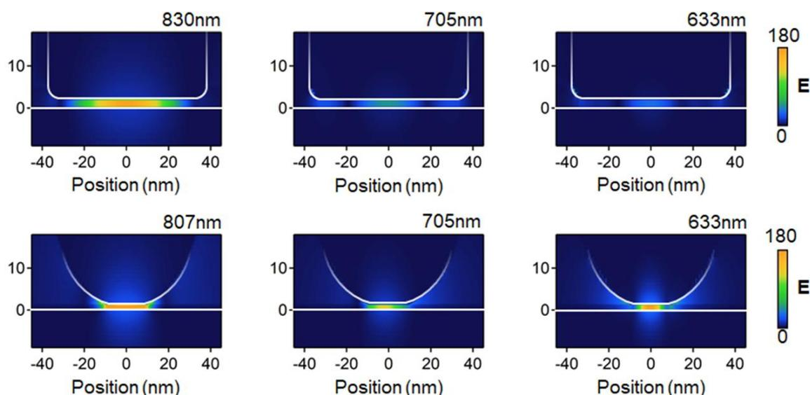
**Fig. S4: Nanoconstruct FDTD simulations.** Simulated near-field maps of the total electric field (E) for NCoM (top row) and NPoM (bottom row) at a resonance position of their modes. The cube size is 75 nm with 5nm edge rounding and the globular nanoparticle is 80 nm with a 20 nm facet size. The gap size is 1.3 nm with a semi-infinite Au mirror underneath.
