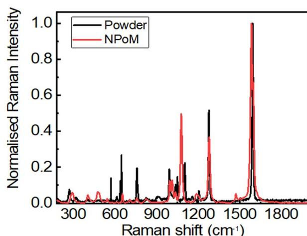
**Fig. S3: Comparison of powder Raman and NPoM SERS spectrum** for an excitation wavelength of 633 nm.
