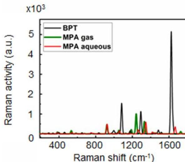
**Fig. S5: DFT simulations within different surrounding medium.** Raman activity is calculated for BPT (black) and MPA (green) considering bond (Au-S) with substrate and gas phase. In addition, Raman activity is simulated for MPA within aqueous solution (red).
