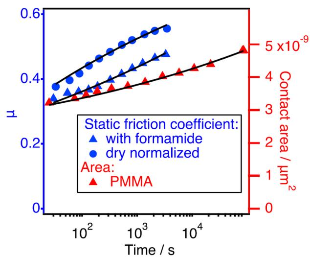
Figure S1: Ageing of the static friction force for PMMA on glass (in blue). All data sets show pronounced ageing: the static friction force increases logarithmically over the duration of the experiment. The black lines are semilogarithmic fits to the data. Red data points depict the growth of the PMMA-on-glass contact area with time as determined from molecular-probe fluorescence images taken during a static ageing experiment, in which the contact is only loaded in the normal direction.
