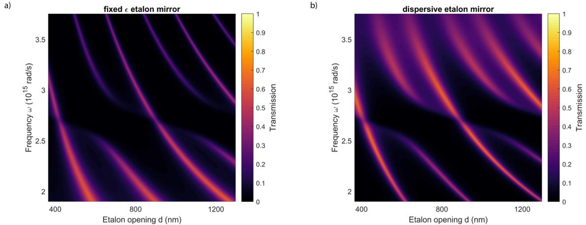
Figure S1: Calculated transmission through a planar Fabry-Pérot cavity-antenna hybrid with pitch 200 nm as a function of etalon thickness and frequency. Calculated with a) dispersionless Au mirrors ( $\epsilon = \sqrt{0.25 + 4.5i}$ ) and b) taking into account the dispersion of the Au mirrors.
