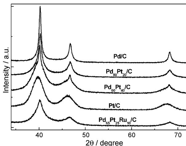
Fig. 1. X-ray diffractograms for PdPt/C and PdPtRu/C catalysts.  $\lambda = 1.54056 \text{ \AA}$  ( $K\alpha$  Cu).
