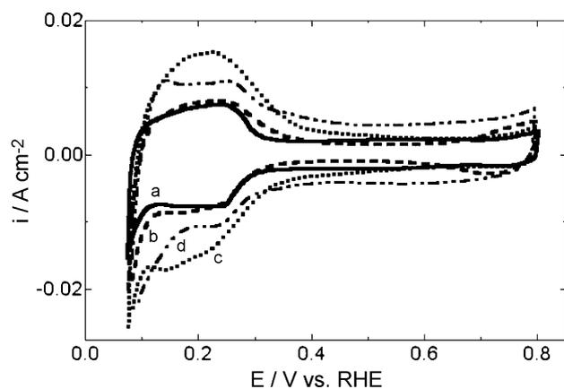
Fig. 4. Cyclic voltammograms for anodes formed by (a) Pd/C, (b) Pd<sub>90</sub>Pt<sub>10</sub>/C, (c) Pd<sub>50</sub>Pt<sub>50</sub>/C and (d) Pt/C catalysts. Nafion<sup>®</sup> 115 membrane;  $T = 27 \pm 2^\circ\text{C}$ ;  $\nu = 50 \text{ mV s}^{-1}$ .
