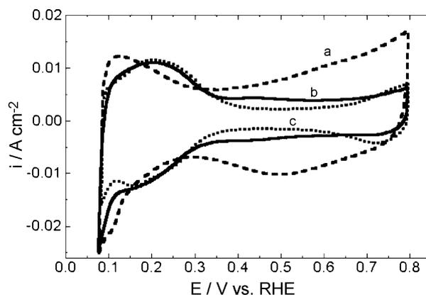
Fig. 5. Cyclic voltammograms for anodes formed by (a) Pd<sub>25</sub>Pt<sub>25</sub>Ru<sub>50</sub>/C, (b) Pd<sub>65</sub>Pt<sub>25</sub>Ru<sub>10</sub>/C and (c) Pd<sub>70</sub>Pt<sub>30</sub>/C catalysts. Nafion<sup>®</sup> 115 membrane;  $T = 27 \pm 2^\circ\text{C}$ ;  $\nu = 50 \text{ mV s}^{-1}$ .
