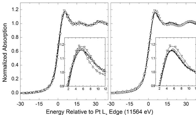
Fig. 2. XANES spectra at the Pt L<sub>3</sub> edge. (□) Pd<sub>80</sub>Pt<sub>20</sub>/C, (○) Pd<sub>60</sub>Pt<sub>40</sub>/C, (△) Pd<sub>50</sub>Pt<sub>50</sub>/C, (▽) Pt/C, (◇) Pd<sub>65</sub>Pt<sub>25</sub>Ru<sub>10</sub>/C, (+) Pd<sub>25</sub>Pt<sub>25</sub>Ru<sub>50</sub>/C, at 200 mV vs. RHE. T = 25 °C.
