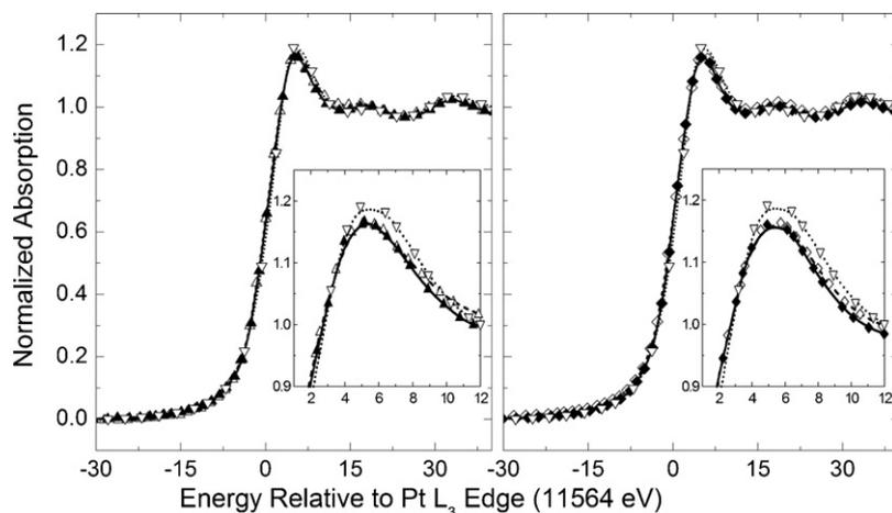
Fig. 3. XANES spectra at the Pt  $L_3$  edge at different potentials vs. RHE. ( $\nabla$ ) Pt/C at 200 mV, ( $\Delta$ ) Pd<sub>50</sub>Pt<sub>50</sub>/C at 200 mV, ( $\blacktriangle$ ) Pd<sub>50</sub>Pt<sub>50</sub>/C at 500 mV, ( $\diamond$ ) Pd<sub>65</sub>Pt<sub>25</sub>Ru<sub>10</sub>/C at 200 mV and ( $\blacklozenge$ ) Pd<sub>65</sub>Pt<sub>25</sub>Ru<sub>10</sub>/C at 500 mV vs. RHE.  $T = 25^\circ\text{C}$ .
