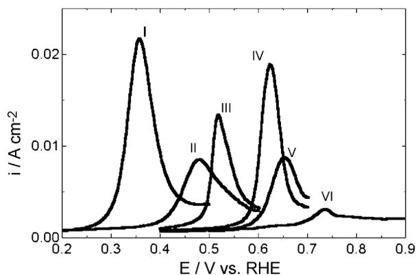
Fig. 6. CO stripping scans for anodes formed by: (i) Pd<sub>25</sub>Pt<sub>25</sub>Ru<sub>50</sub>/C, (ii) Pd<sub>65</sub>Pt<sub>25</sub>Ru<sub>10</sub>/C, (iii) Pt/C, (iv) Pd<sub>60</sub>Pt<sub>40</sub>/C, (v) Pd<sub>90</sub>Pt<sub>10</sub>/C and (vi) Pd/C. Electrosorption at 100 mV (vs. RHE). Nafion® 115 membrane;  $T = 85^\circ\text{C}$ ;  $\nu = 10 \text{ mV s}^{-1}$ .
