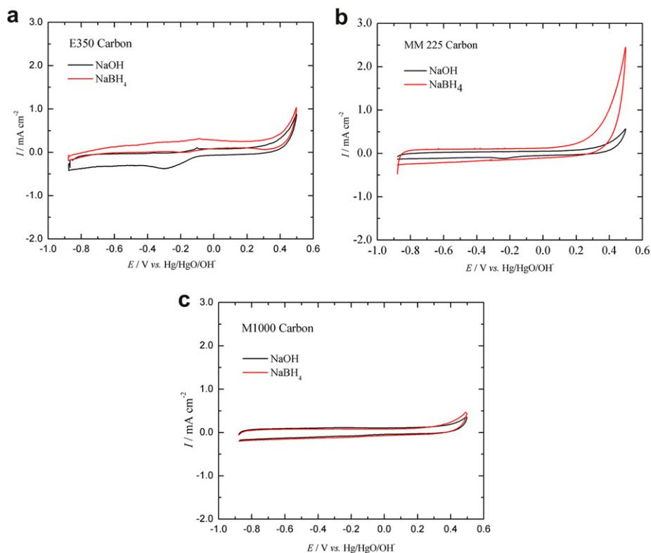
**Fig. 3.** Cyclic voltammograms plotted at 5.0 mV s<sup>-1</sup> in the absence of any O<sub>2</sub> in solution for the three bare carbon substrates in the presence and absence of 10<sup>-3</sup> mol L<sup>-1</sup> NaBH<sub>4</sub> in the 1.0 mol L<sup>-1</sup> NaOH supporting electrolyte. Electrode geometric area: 0.196 cm<sup>2</sup>.
