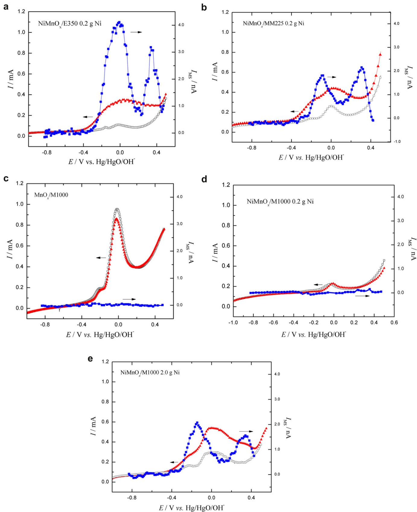
**Fig. 4.** Faradaic and ionic currents for  $\text{H}_2$  formation ( $m/z = 2$ ) obtained in DEMS experiments during CV (positive-going scan) of borohydride electro-oxidation reaction catalyzed by the different investigated  $\text{MnO}_x$ -based electrocatalysts, in the presence (triangles) and absence (squares) of  $10^{-3} \text{ mol L}^{-1} \text{ NaBH}_4$  in the  $1.0 \text{ mol L}^{-1} \text{ NaOH}$  supporting electrolyte. Scan rate of  $5.0 \text{ mV s}^{-1}$ .
