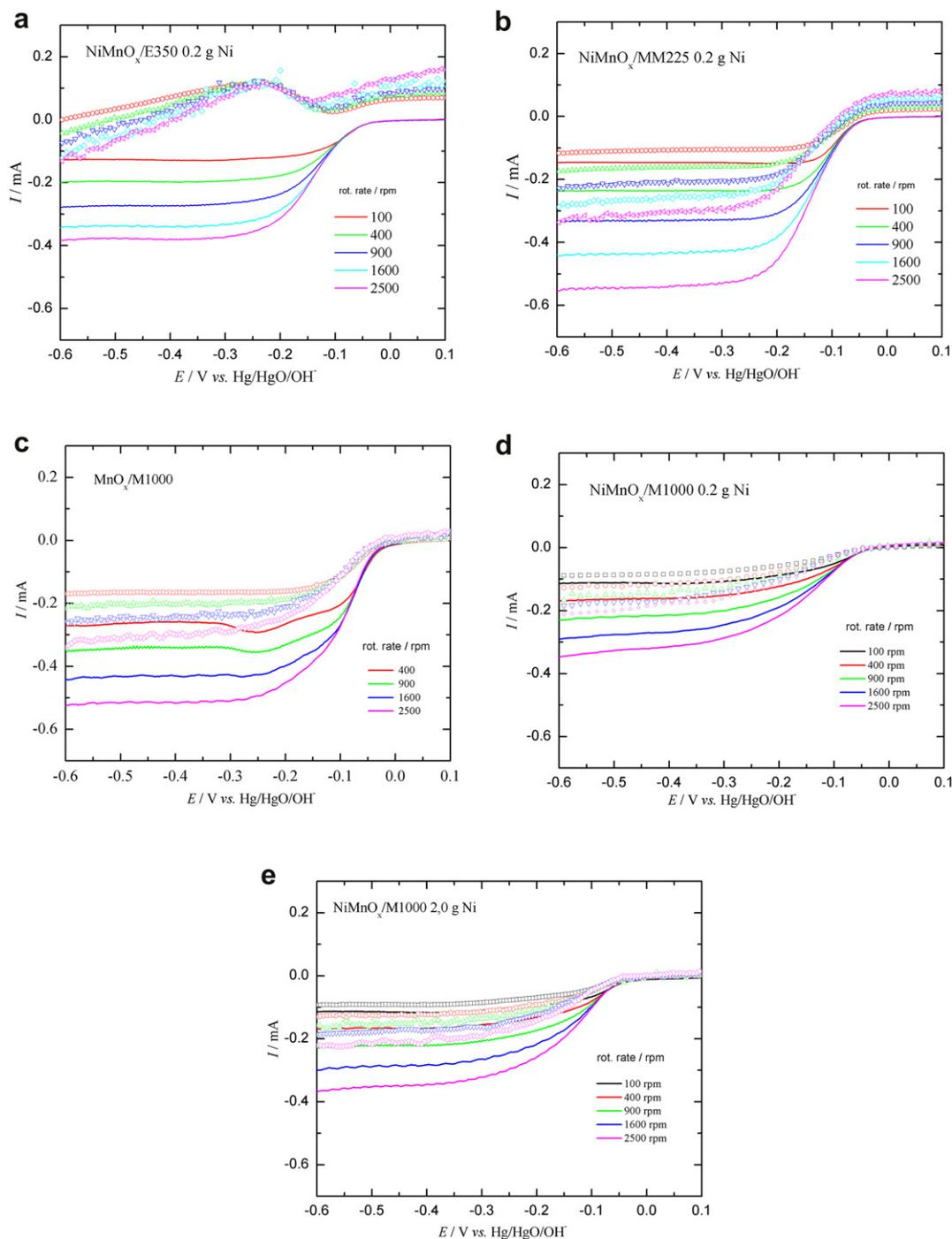
**Fig. 2.** Oxygen reduction reaction (ORR) voltammograms ( $5.0 \text{ mV s}^{-1}$ ) obtained on  $\text{MnO}_x$ -based electrocatalysts in the RDE setup. (symbol) in  $1.0 \text{ mol L}^{-1} \text{ NaOH} + 10^{-3} \text{ mol L}^{-1} \text{ NaBH}_4$  and (lines) in  $1.0 \text{ mol L}^{-1} \text{ NaOH}$ . Electrode geometric area:  $0.196 \text{ cm}^2$ .
