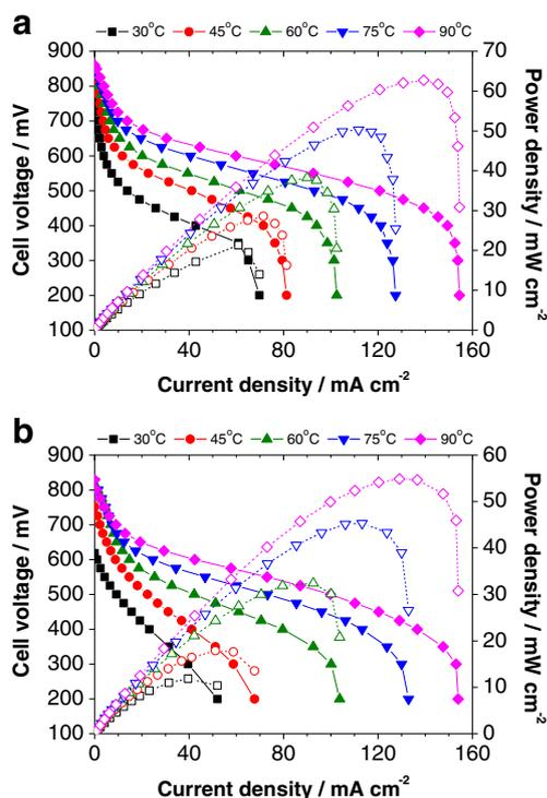
**Fig. 5** Cell potential and Power density versus current densities for alkaline single cells operating at different temperatures for the different cathode materials: **a** Pt/C and **b** NiMnO<sub>x</sub>/C
