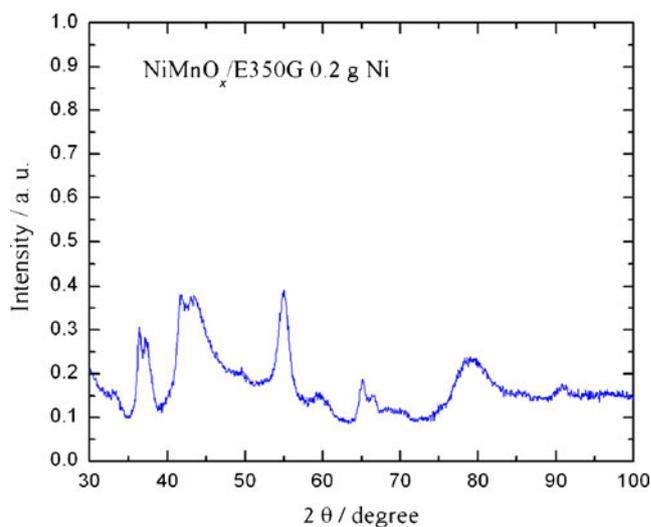
**Fig. 1** DRX pattern of the synthesized NiMnO<sub>x</sub>/C catalyst
