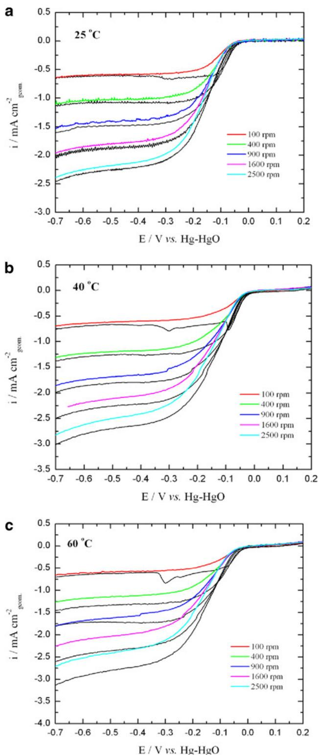
**Fig. 4** Voltammograms toward oxygen reduction reaction NiMnO<sub>x</sub>/C electrocatalyst in presence and absence of ethanol at different temperatures. *Black traces*: in pure 1 mol L<sup>-1</sup> NaOH. *Colored traces*: in the presence of 0.1 mol L<sup>-1</sup> ethanol
