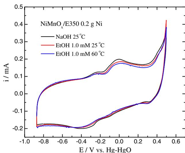
**Fig. 3** Cyclic voltammograms for NiMnO<sub>x</sub>/C catalyst obtained at 0.01 V s<sup>-1</sup> in 1.0 mol L<sup>-1</sup> NaOH and 0.1 mol L<sup>-1</sup> ethanol at different temperatures
