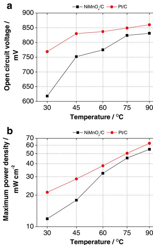
**Fig. 6** **a** Open circuit voltage and **b** fuel cell maximum power density for the different cathode catalyst materials at the studied temperatures
