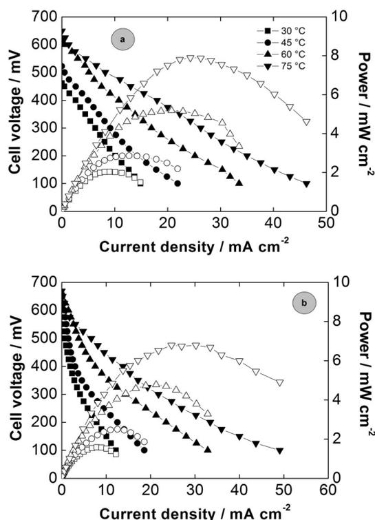
**Figure 5.** Polarization curves at different temperatures of the catalysts in the single fuel cell. a) Au/C and b) AuAg/C with no backpressure (4 mol L<sup>-1</sup> KOH and 1 mol L<sup>-1</sup> glycerol at 1 mL min<sup>-1</sup> and an oxygen flow of 0.1 L min<sup>-1</sup>). Metal loading in the anode was 2 mg cm<sup>-2</sup>, and platinum loading in the cathode was 1 mg cm<sup>-2</sup>.
