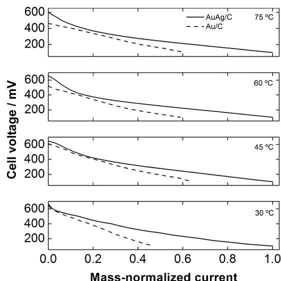
**Figure 6.** Mass-normalized polarization curves for comparison of Au/C and AuAg/C in terms of mass of gold.
