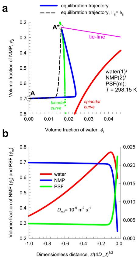
**Figure 5.** (a) Transient equilibration trajectory A–A\* water/NMP/PSF casting film. (b) Transient volume fraction profiles in the casting solution, as a function of the dimensionless distance coordinate  $z/\sqrt{4D_{\text{ref}}t}$ . Further calculation details and data inputs are provided in the Supporting Information accompanying this publication.
