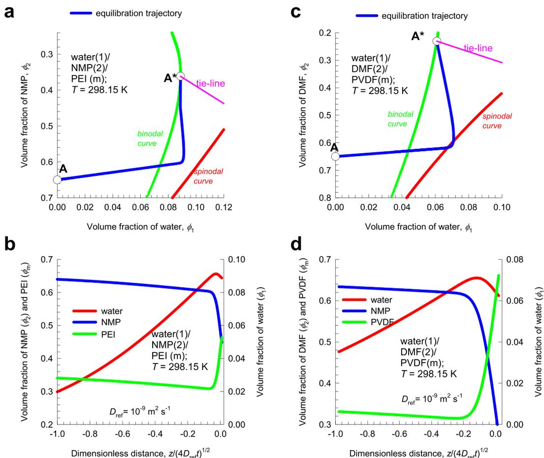
**Figure 6.** (a, b) Transient equilibration in the water/NMP/PEI casting film. (c, d) Transient equilibration in the water/DMF/PVDF casting film. Further calculation details and data inputs are provided in the [Supporting Information](#) accompanying this publication.
