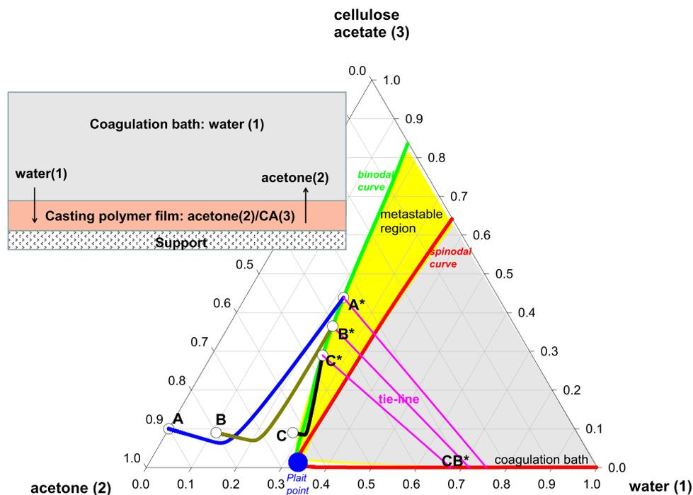
**Figure 1.** Transient equilibration trajectories A–A\*, B–B\*, and C–C\* during the immersion precipitation process for membrane preparation. These trajectories were determined from simulations using the starting compositions A, B, and C in the polymer casting film. Further calculation details and data inputs are provided in the [Supporting Information](#) (SI) accompanying this publication.
