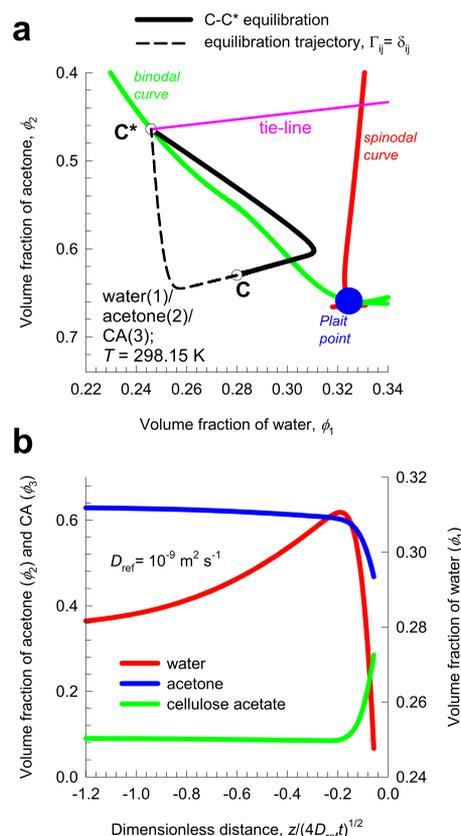
**Figure 4.** (a) Transient equilibration trajectory C–C\* in the water/acetone/casting film. The dashed lines represent simulation results when the simplification  $\Gamma_{ij} = \delta_{ij}$ , the Kronecker delta, is invoked. (b) Transient volume fraction profiles in the casting solution, as a function of the dimensionless distance coordinate  $z/\sqrt{4D_{ref}t}$ . Further calculation details and data inputs are provided in the Supporting Information accompanying this publication.
