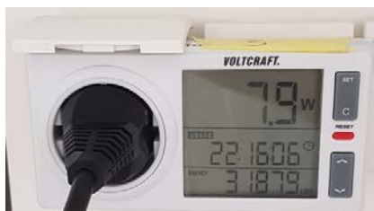
Figure S10. Amperometer used to determine the electricity consumption.
