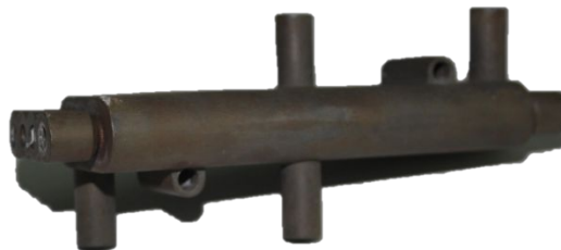
Figure S1. Images of the two 3D-printed in Ti 6Al-4V devices a) the direct contact (DC) device, b) the heating/cooling jacket (HCJ) device.
