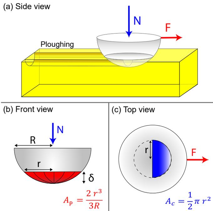
**Figure 3.1:** Schematic representation of the ploughing experiment. **a)** Side view: Normal ( $N$ ) and frictional ( $F$ ) forces which act on the sliding hemisphere. **b)** Front view: The hemisphere with radius  $R$ , where the ploughing cross section  $A_P$  (red) can be calculated using the track radius  $r$ . **c)** Top view: The hemisphere with the projected area of contact  $A_c$  (blue).
