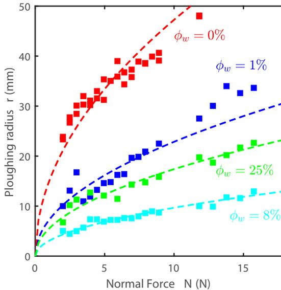
**Figure 3.5:** Ploughing radius  $r$  as a function of normal force  $N$  for various water volume fractions. The squares represent the experimental data and the dashed lines reflect the model ( $r = \sqrt{\frac{N}{\frac{1}{2}\pi P_h(\phi_w)}}$ ) based on the penetration hardness. The radius increases with the normal force and has a minimum for  $\phi_w = 8\%$ . Note that the nonmonotonic behaviour of the track radius for increasing water content holds over the full domain of normal forces.
