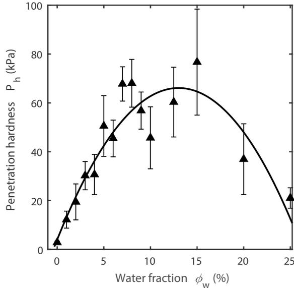
**Figure 3.4:** Penetration hardness  $P_h$  as a function of water volume fraction  $\phi_w$ . The error bars represent the standard deviation. The solid line describes the data based on a first-order increase due to liquid bridge formation and an exponential decrease based on the coalescence of these liquid bridges.
