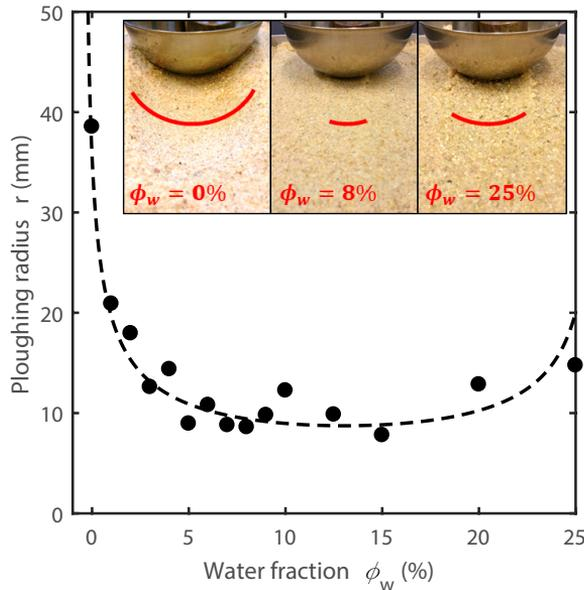
**Figure 3.3:** Ploughing radius  $r$  as a function of water volume fraction  $\phi_w$  for a fixed normal force of  $N = 7.9$  N. Like the friction coefficient, the ploughing track width (black circles) evolves nonmonotonically with the water content, also shown based on the ploughing model (dashed line,  $r = \sqrt{\frac{N}{\frac{1}{2}\pi P_h(\phi_w)}}$ ). The inset shows images of the experiments for  $\phi_w = 0, 8$  and  $25\%$  with red lines highlighting the ploughing tracks.
