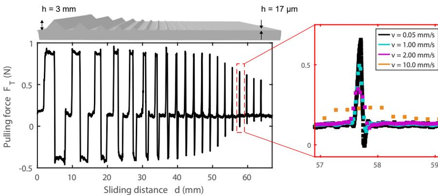
**Figure 6.7:** Pulling force  $F_T$  as a function of the sliding distance  $d$  for a sawtooth patterned ( $\theta = 45^\circ$ ) surface fabricated in aluminium with a stepwise decreasing height  $h$ . The sliding speed is set at  $v = 0.05$  mm/s for an imposed gravitational load of  $F_G = 0.72$  N. On the right, the measured pulling force for sliding over a single sawtooth pattern is given for various sliding speed.
