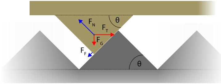
**Figure 6.5:** Schematic illustration, including a force balance, for sliding two sawtooth patterned surfaces with patterning angle  $\theta$  over each other.  $F_G$  is the gravitational force,  $F_N$  the normal force,  $F_F$  the friction force and  $F_T$  the horizontal pulling force.
