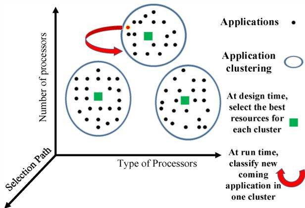
Figure 1. Clustering at design time and classification at run time.
