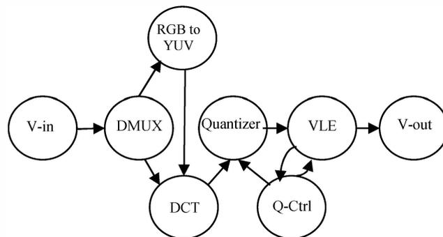
Figure 2. KPN Model for an MJPEG encoder.
