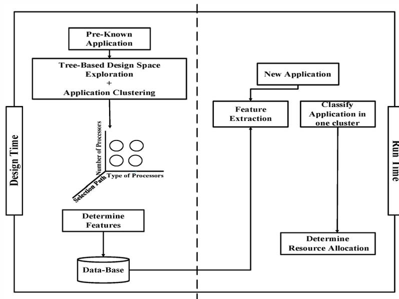
Figure 3. Workflow of proposed run-time mapping approach
