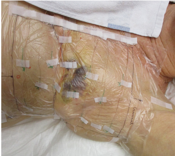
Figure 1. The standard of care thermometry during hyperthermia treatments at the Amsterdam University Medical Centers. Multiple seven point thermocouples probes are distributed over the skin surface of the target area. To allow accurate positioning and for hygienic reasons a 10 \mu\text{m} high density polyethylene plastic foil is positioned on the chest wall of the patient and the thermocouple probes are placed on the foil.
