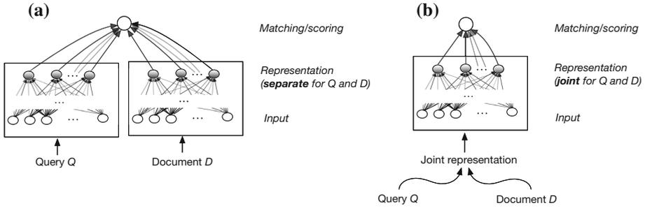
**Fig. 8** Two basic neural architectures for scoring the relevance of a TTU pair, query and document for illustrative purposes. **a** Representation Based, **b** Interaction Based. This figure is inspired by Figure 1 in Guo et al. (2016a)
