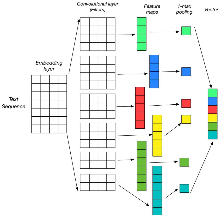
**Fig. 2** One-dimensional CNN with only one convolution layer (six filters and six feature maps), followed by a 1-max-pooling layer
