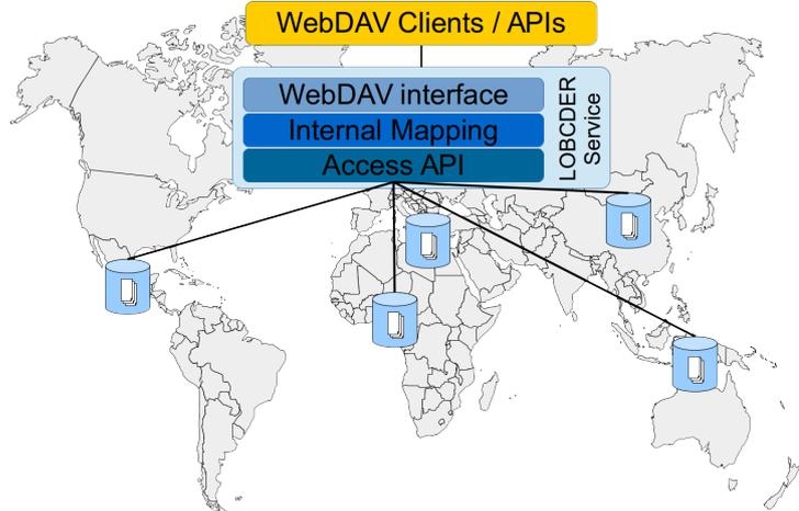
**Fig. 1.** LOBCDER’s architecture. The top layer is a WebDAV repository, the middle layer maps the physical files to a logical file system and the bottom layer provides transparent access to a variety of infrastructures.
