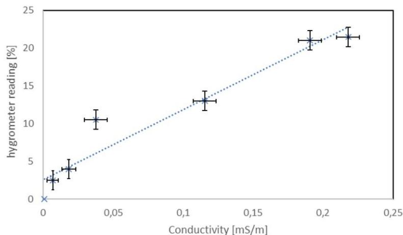
**Fig. S1 Conductivity calibration**
