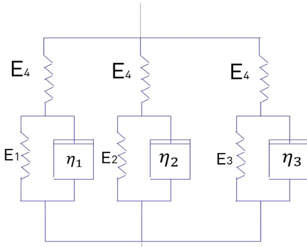
**Figure S4 Rheological model used to describe the stress relaxation curves.** The ideal solid elements are represented by springs (with an associated Young modulus  $E$ ), and the ideal viscous elements by dashpots (with viscosity  $\eta$ )
