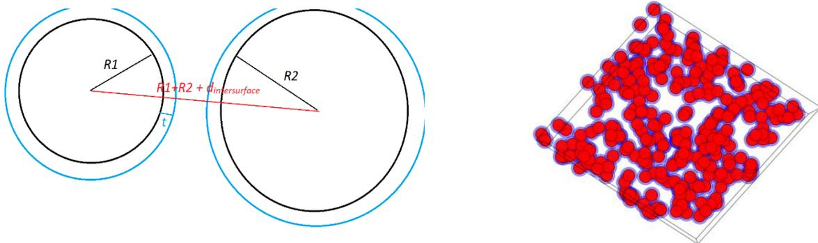
**Figure S2 Schematic of the simulation principle.** (left) When the center-to-center distance is smaller than  $R_1 + R_2 + 2t$ , where  $t$  is the water layer thickness, the water layers overlap. (right) Reconstruction of the simulated system showing the spherical inclusions (red dots) and their shells modelling the water layers (blue).
