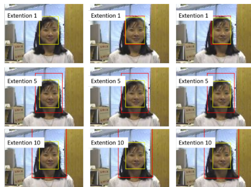
Figure 1: Predictions from ECO [6] on an artificially extended video created from OTB50 data (red box: tracker prediction, yellow box: ground truth prediction). Model decay is prevalent here although the appearance variation remains intact. Due to heavy updating involved, model decay is noticeable from very early stages itself, even for clearly visible target objects moving slowly.
