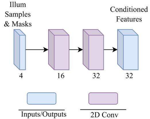
Figure 2. The architecture for the illumination processing head is shown. The input is the sparse illumination samples and the corresponding masks, concatenated channel wise (3+1 channels). This is passed through two convolution layers, which squeezes and subsequently expands the channels of the outputs, thus conditioning the features down to the useful features in an end-to-end manner.
