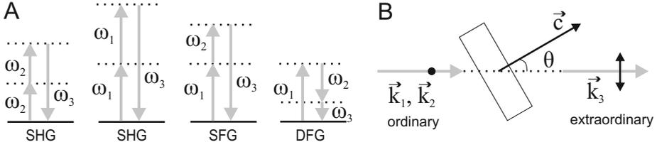
FIGURE 3.1. (A) Energy level description of second-order frequency conversion processes induced by light fields at  $\omega_1$  and  $\omega_2$ : second harmonic generation (SHG), sum-frequency generation (SFG) and difference-frequency generation (DFG). Dashed lines indicate virtual states. (B) Geometry of phase-matching for sum-frequency generation in a negative ( $n_e < n_o$ ) uniaxial crystal (type I). The dot and double-sided arrow indicate the polarization directions of the fields.
