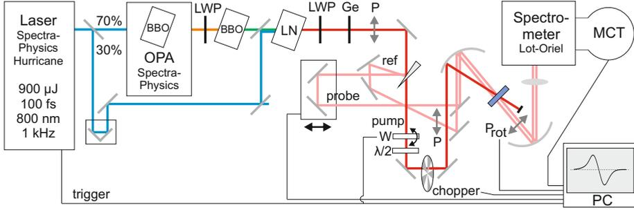
FIGURE 3.2. Schematic of the single-color pump-probe setup described in the text (not to scale). BBO:  $\beta$ -bariumborate crystal, LN: lithiumniobate crystal, LWP: long wave pass filter, Ge: Germanium filter, P: polarizer,  $P_{rot}$ : rotating polarizer, W: wobbler (optional),  $\lambda/2$ : half-wave plate, MCT: Mercury-Cadmium-Telluride detector. The colored lines indicate light beams, while the thin black lines indicate electronic signals.
