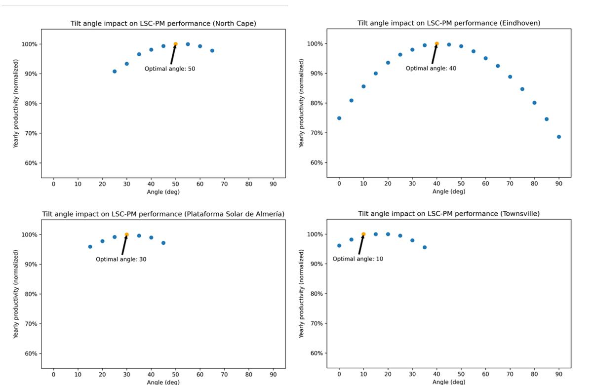
Figure 9 Angle optimization for North Cape, Eindhoven, Plataforma Solar de Almería and Townsville.
