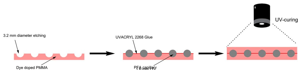
Figure 1 Construction method scaled-up LSC-PM
