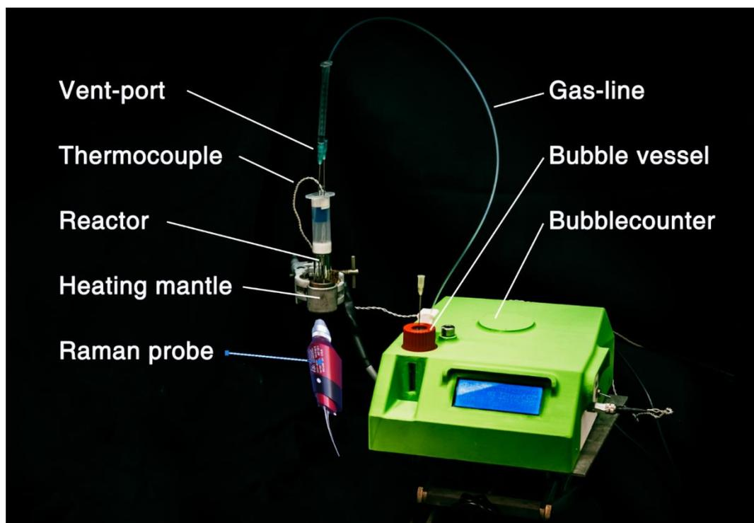
**Figure S3** The bubble counter coupled with operando raman set-up for mechanistic and kinetic experiments. The bubblecounter both counts produced gas bubbles and controls the heating mantle. Reactor and bubble vessel are connected via a gas line; inert conditions are kept as the bubble vessel functions as an airlock.
