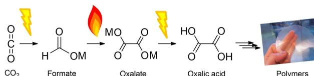
**Figure 1.** "OCEAN" process for CO<sub>2</sub> utilization via electrochemical reduction to formate, thermal formate coupling to oxalate, electrochemical oxalate acidification, and polymer production from oxalic acid and its derivatives.
