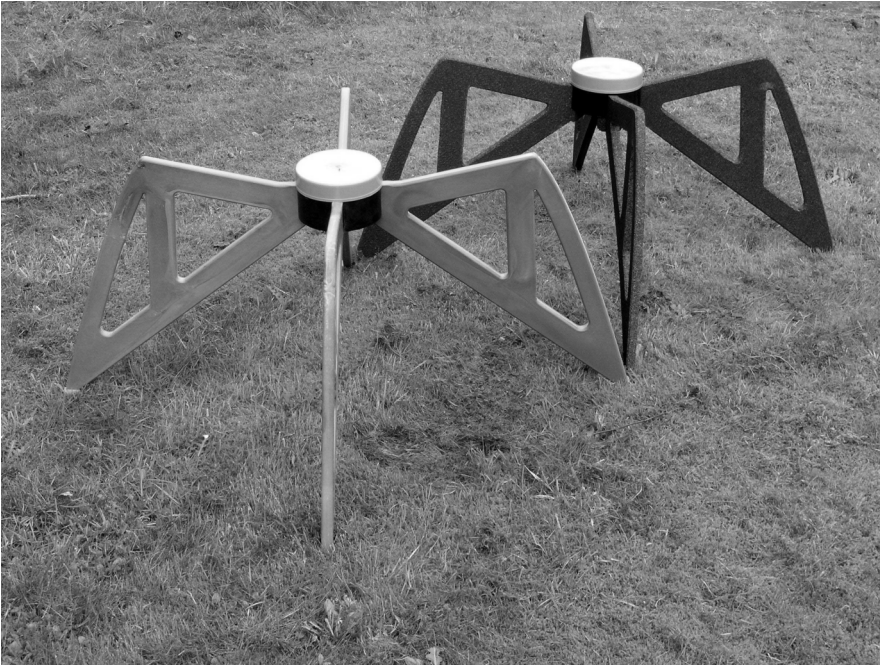
Figure 1.2: A close-up of two High Band Antennas.
