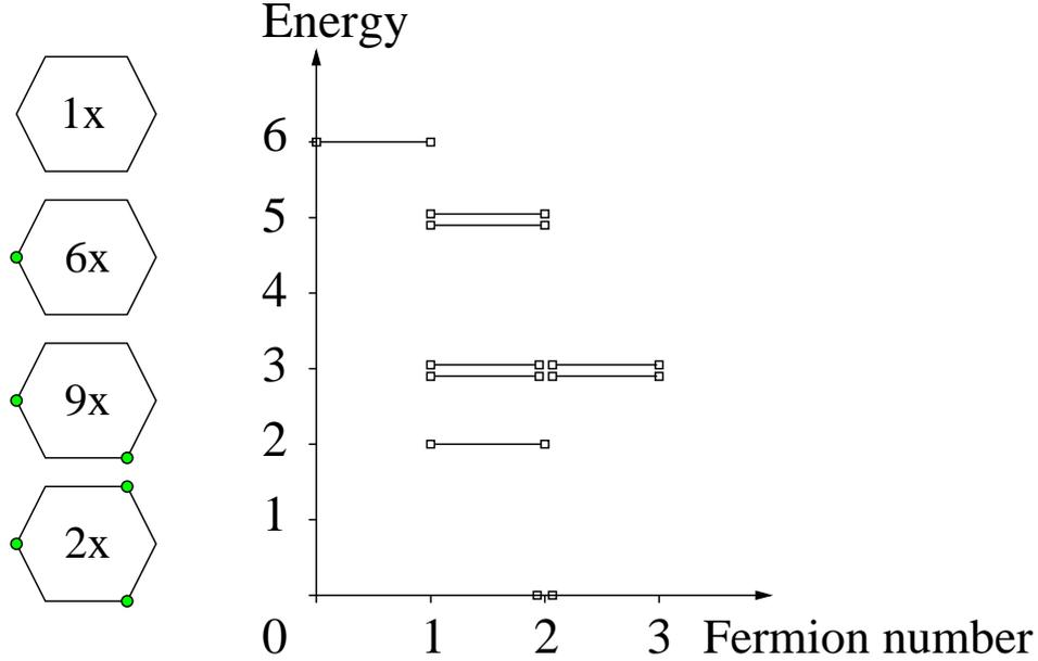
**Figure 2.1:** On the left we show the 6-site chain and the possible configurations of hard-core fermions on this lattice. The numbers give the number of possible configurations with a given number of fermions. On the right we show the spectrum, energy versus fermion number, of the 6-site chain.
