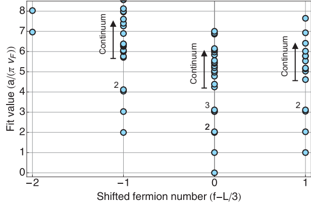
(b) The numerically fitted values of the energy are plotted versus the shifted fermion number \tilde{f} \equiv f - L/3 for chains of length L = 3j . The fit values are obtained by fitting the numerically obtained energies as a function of the chain length L with the function f(L) = a/L + b/L^2 + c/L^3 . The energy is then given by E = a/(\pi v_F) . The labels indicate the number of overlapping data points.
