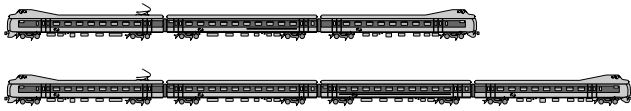
Figure 4: This figure illustrates two single-deck rolling-stock units with three and four carriages, respectively. A train consists of several of these units.
