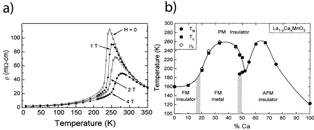
Fig. 2.1 (a) The colossal magnetoresistance effect of  $\text{La}_{0.75}\text{Ca}_{0.25}\text{MnO}_3$ . (b) The phase diagram of calcium doped manganites. Taken from Schiffer et al. [22].
