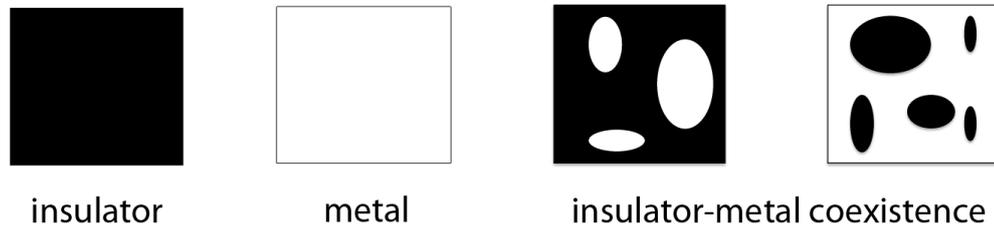
Fig. 2.2 A simple model of 2D phase separation. Left: conventional materials are either an insulator (black), a metal (white), or a semiconductor. Right: in phase separated systems, more than one electronic phase (insulator and metal) coexists. Conductivity is only possible if a percolative metallic pathway (white) connects two edges of the system.
