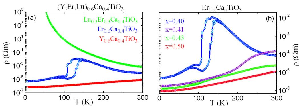
Fig. 2.8 Transport measurements of  $R_{1-x}Ca_xTiO_3$ . The left graph plots the temperature dependent resistivity measurements for different R cations (Y, Er, Lu), for which the ionic radius decreases along this series. The data in the left panel show a tilting tuned metal insulator transition. On the right side, the graph shows explicitly the doping tuned metal insulator transition with fixed R ion (Er). The metal-insulator transition exhibits a thermal hysteresis. Data from Ref. [23].
