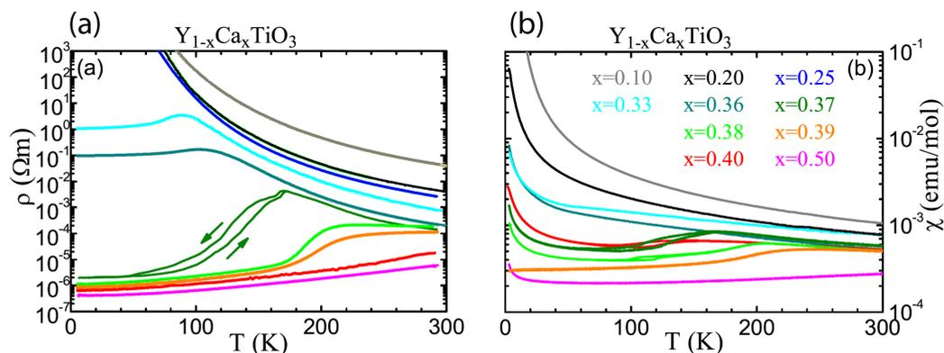
Fig. 2.5 (a) The temperature dependence of the resistivity, (b) the susceptibility of the (YCa)TiO<sub>3</sub> system. Data from A. C. Komarek [16].
