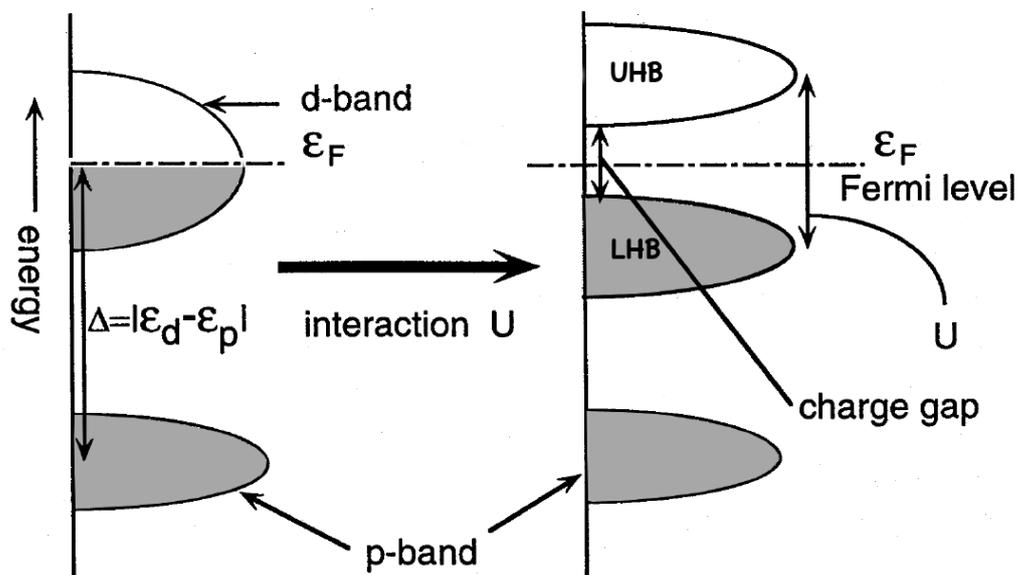
Fig. 2.4 Taken from Ref. [20]. A schematic illustrating the effects of switching on the electron-electron interaction  $U$ . The previous metal with half filled  $d$  band (left panel) becomes a Mott-Hubbard insulator (right panel) as the  $U$  splits the  $d$  band into upper Hubbard band (UHB) and lower Hubbard band (LHB) with charge gap, in which the Fermi level lies.
