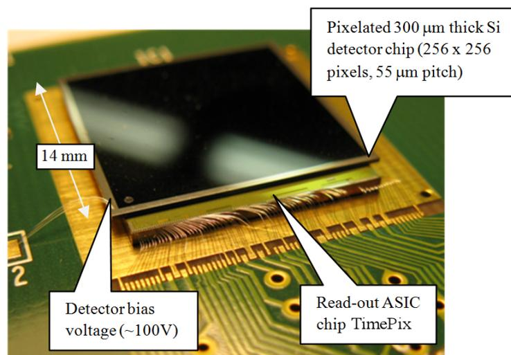
Fig. B.1 Picture of the Timepix detector. An application-specific integrated circuit (ASIC) is attached to the silicon sensor with Indium bump-bonding. Adopted from the Timepix website.
