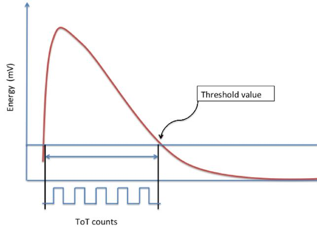
Fig. B.3 The counting logic of the ToT mode. The pre-amplifier converts the collected charges into a standard pulse shape, whose integral is proportional to this charge and accordingly proportional to the photon energy. The signal is the number of cycles of a 40 MHz internal clock that are counted while the input pulse is over the preset threshold voltage.
