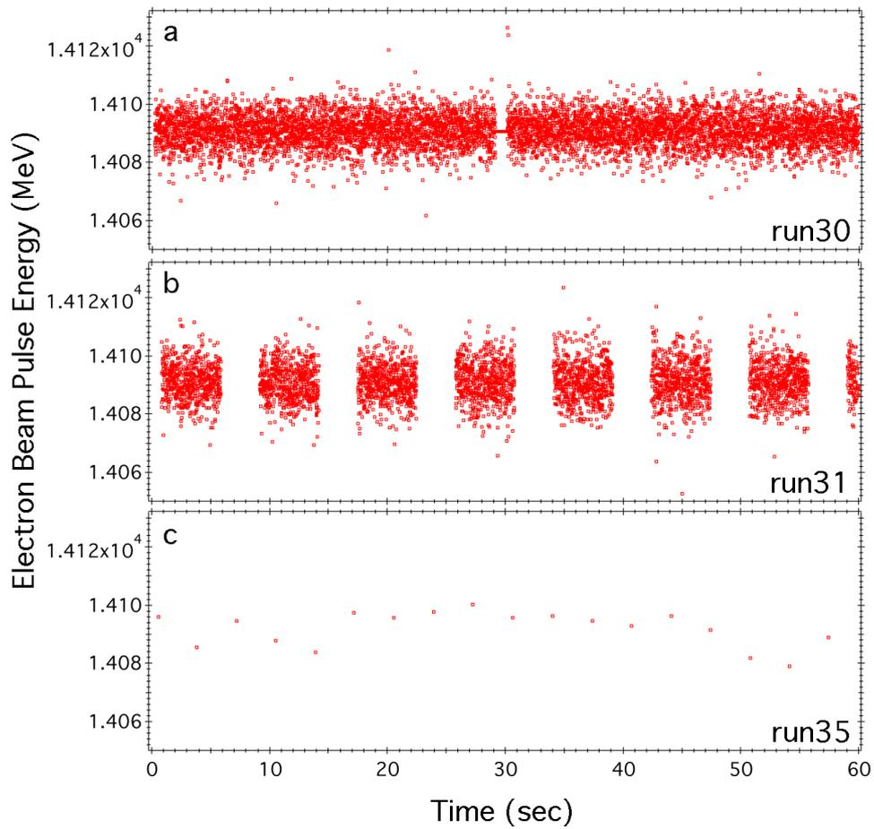
Fig. C.2 Examples of the electron beam pulse energy for the three LINAC operation modes used in our experiments: (a) 120 Hz continuous mode, (b) burst mode, (c) one shot mode. The nominal energy of the electron beam pulse energy is 14091 MeV
