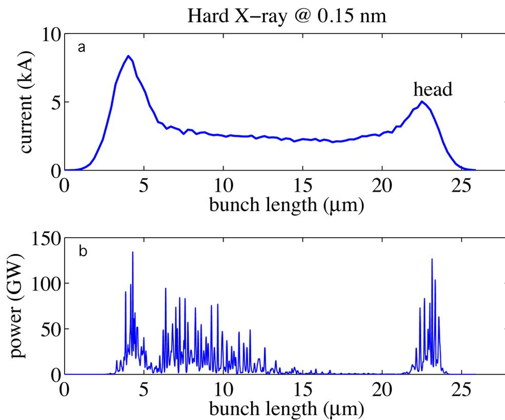
Fig. C.1 (a) The current profile of a compressed electron bunch with 250 pC charge. (b) The power profile of the resulting X-ray pulse train. Taken from LCLS FAQ web page [25].
