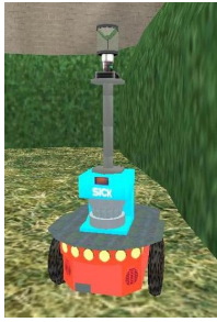
Fig. 7: OmniP2DX, with the omnica sensor high above the Sick laser range scanner.
