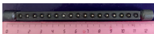
Figure 5. 3D-printed internal part of the SLIT device with O-rings and a monolith created in-situ . Indicated scale is in cm.
