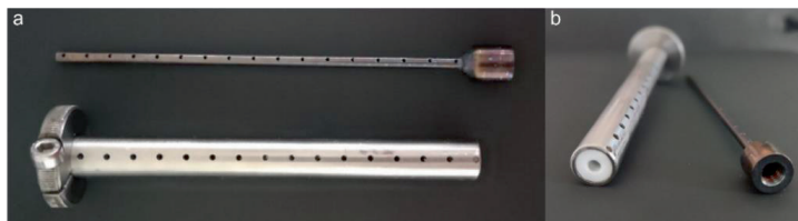
Figure 2. a) top view and b) axial view of the 3D-printed metal version of the internal part of the TWIST with through holes (titanium alloy, Ti-6Al-4V; appearing dark coloured) and the stainless-steel metal rod with Teflon sleeve and through holes (external part) used in some of the experiments described in this paper.
