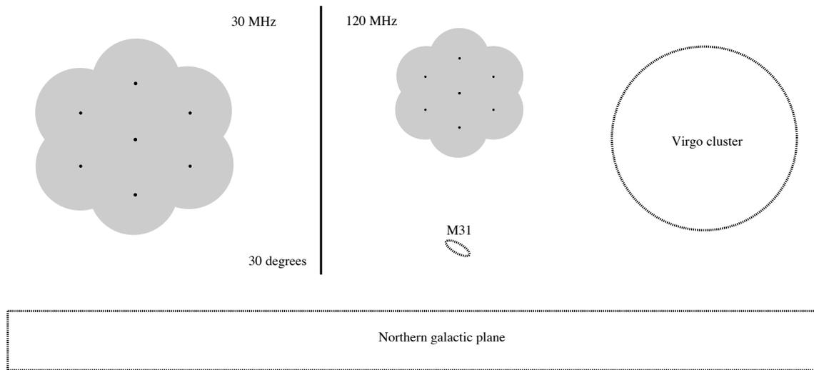
**Figure 2:** An example of a Radio Sky Monitor (RSM) observing modes. In this example a hexagonal pattern is traced out using seven beams and an offset between pointing centres of  $\text{FWHM}/\sqrt{2} = 6.4$  and  $3.7$  degrees at 30 and 120 MHz respectively. The approximate angular size on the sky of M31, the Virgo cluster and the northern galactic plane are indicated for comparison. The angular resolution within these fields of view depends upon the longest baselines used – see Table 1.
