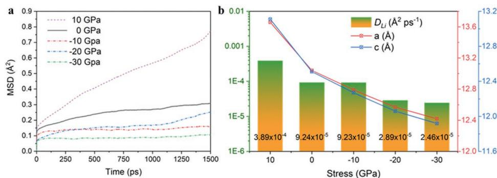
**Figure 2.** a) Mean square displacement (MSD) versus time for LLZTO at 300 K and b) lithium diffusion coefficients ( $D_{Li}$ ), and lattice parameters  $a$  and  $c$  (b is equal to  $a$ ) for LLZTO under tensile (10 GPa) stress, no stress (0 GPa), and compressive (−10, −20, and −30 GPa) stress.
