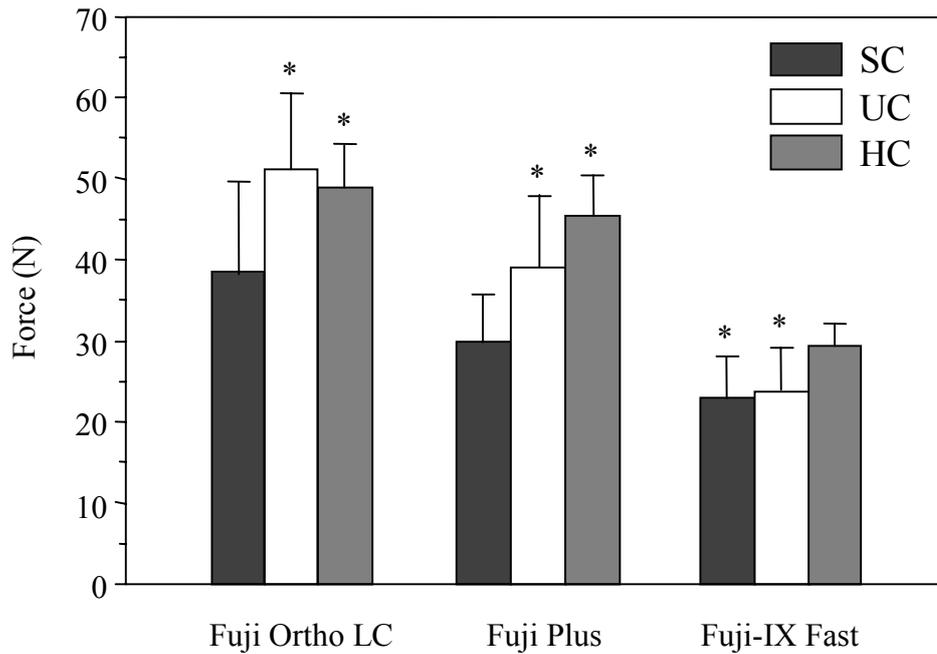
**Figure 3.3** Mean tensile fracture force and standard deviation determined 15 minutes after the start of the bonding procedure. HC = heat cure, UC = ultrasonic cure and SC = standard cure. Values within a group that are not significantly different from each other are marked with an asterisk ( $P > 0.05$ ).
