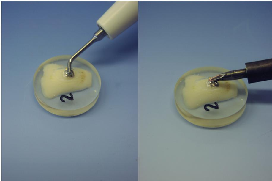
**Figure 3.1** Application of ultrasound (a) and heat (b) to the bracket. Ultrasonic energy was applied by holding the tip slightly above the wings (no direct contact) with a liquid medium between the tip and bracket. Heat was applied by placing the tip of the soldering iron directly on the wings of the bracket.
