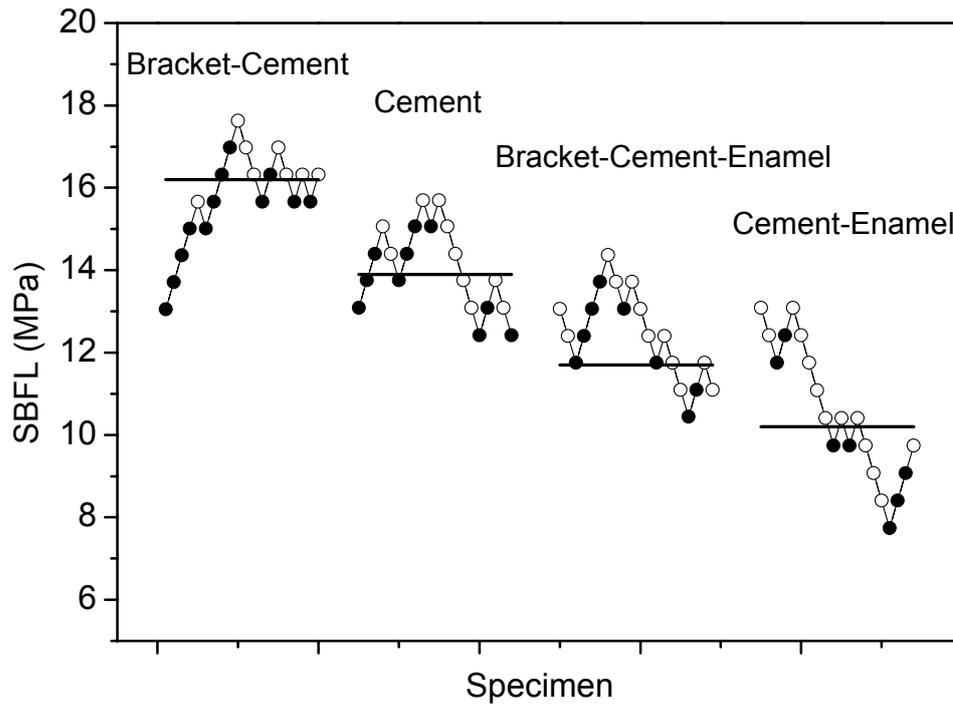
**Figure 6.3** This graph shows the staircase results of Fuji Ortho LC for the four variables. Black dots indicate that the specimen did not fail whilst the white dots represent failure. From these results the SBFLs were calculated which are represented in the graph by the black lines.
