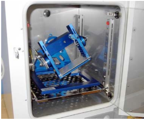
Fig. 7 Desktop RPM in a standard incubator
