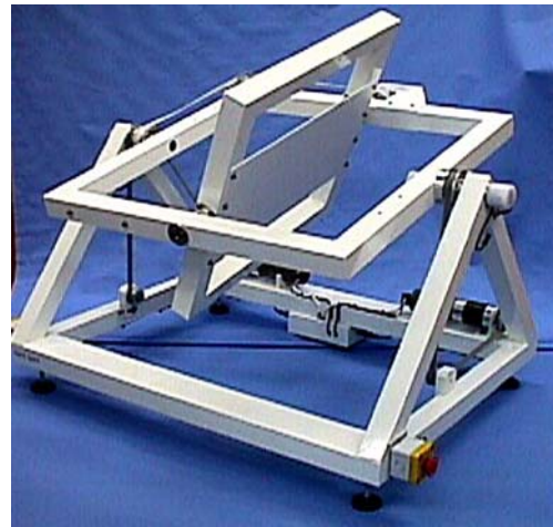
Fig. 2 RPM with two independently driven perpendicular frames
