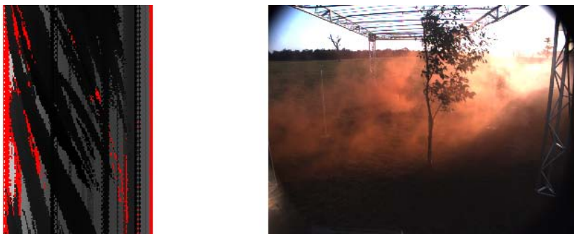
Fig. 3. Snapshot of the data from Peynot et al. [11]. On the left laser range finder readings in a smoky environment. The x-axis is measurement angle, y-axis is time. The darker the color, the shorter the reading is. Red pixels indicate an error code was returned by the laser range finder. The vertical black lines indicate static obstacles. The diagonal black stripes indicate dynamic smoke. On the right the corresponding visual is shown.
