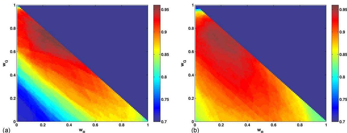
Fig. 4. (Color online) Plot of the correlation coefficients of the weighted Euclidean distance with respect to the human observer (psychophysical data). Only the dependency on weight coefficients  $w_R$  and  $w_G$  are shown here;  $w_B$  follows from  $w_B=1-w_R-w_G$ . Left, the results of experiments using the hyperspectral data are demonstrated; right, results of the experiments with the RGB images.
