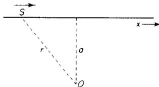
Figure 1. An observer  $O$  at a distance  $a$  from a line on which a source  $S$  moves with speed  $v$ . The projection of  $O$  on the  $x$ -axis is the zero reference point.
