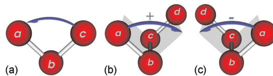
FIG. 1. The bend angle  $\theta$  (a) defined by the angle formed by atoms a-b-c and the dihedral angle  $\phi$  defined by the angle between the planes formed by atoms a-b-c and b-c-d. A positive dihedral angle (b) and a negative dihedral angle (c) are shown.
