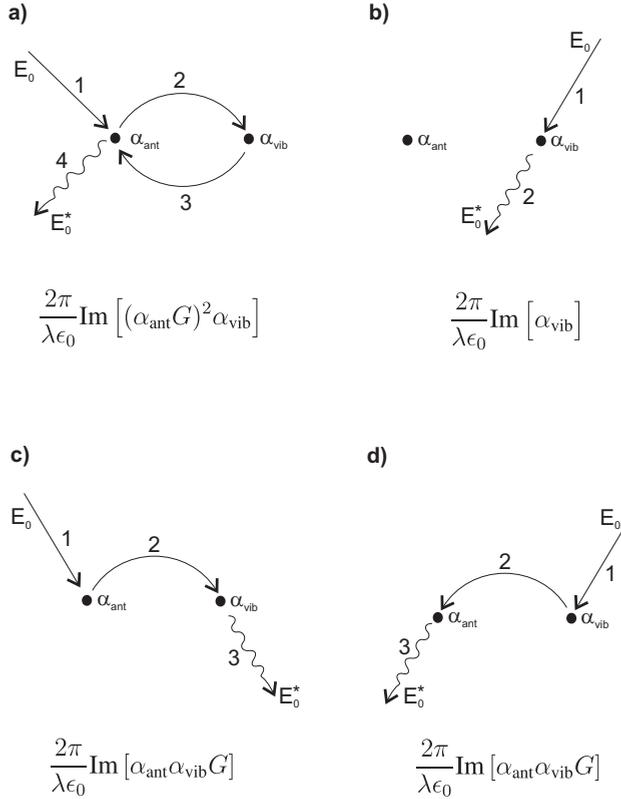
FIGURE 6.3. Scattering diagrams representing the different terms in the expansion from Eq. (6.9). (a) Diagram representing the leading term in the expansion ( $n = 1$  in the first summation symbol). (b) Diagram representing the leading term ( $n = 0$ ) of the second summation symbol. This interaction process represents the direct interaction of the light with the vibrational dipole. (c,d) Scattering diagrams that are grouped together under the third summation symbol of Eq. (6.9).
