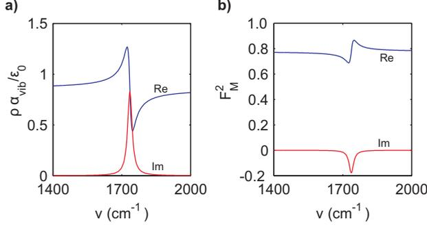
FIGURE 6.10. a) Plot of the vibrational polarizability of PMMA that follows from the experimental permittivity. b) Plot of the factor  $F_M^2$  assuming the experimental polarizability of PMMA and a depolarization factor  $L$  of 0.49.
