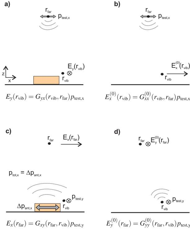
FIGURE 6.12. Diagrams for computing the element  $f'_{xy}$ . In these diagrams the far-field source is placed in such a way that the nanoantenna is illuminated under a slight angle  $\theta$ . We have defined a secondary coordinate system with the  $z'$  axis parallel to the  $k$  vector of the illumination; the  $x'$  axis is perpendicular to this direction and parallel to the electric field of the source dipole.
