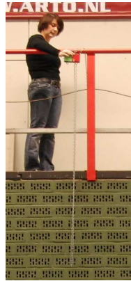
Figure 4. Dropping two wooden blocks simultaneously from a height of a few meters, while one of the blocks is chained and the other is in free fall.
