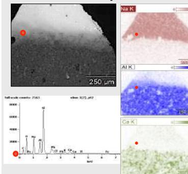
Top left: SEM-EDS image of test sample (JEOL 5910LV, tile 25% CaCO<sub>3</sub> clay), glaze-fired 1000°C; right: Na, Al and Ca elemental mapping collected at 20.0 kV; bottom left: SEM-EDS spectra of interface region. Analysis Ineke Joosten (RCE)
