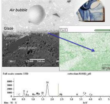
Top left: SEM-EDS image of a sample taken from the tile; Right: Ca elemental map collected at 20.0 kV; bottom: EDS spectra of interface region. Analysis Luc Megens (RCE)
