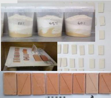
Top: the clay mixes containing various CaCO<sub>3</sub> percentages; middle: Firing of test samples; bottom: colour and shrinkage tests of clay mixes with 20 – 60% CaCO<sub>3</sub> fired at 950°C, sample (a) was re-fired at 1100°C.
