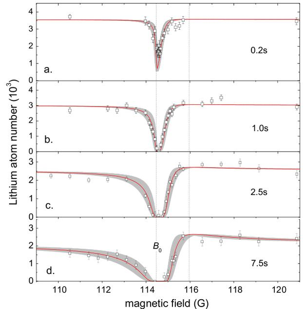
FIG. 2 (color online). Measurement of the Feshbach resonance width (explanation in text). The solid (red) line indicates the best fit obtained for  $B_0 = 114.47(5)$  G and  $\Delta B = 1.5(5)$  G. The gray shaded area indicates the combined error in  $B_0$  and  $\Delta B$ .
