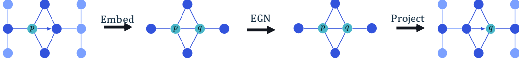
Figure 6: Local NGN message passing with an equivariant graph network kernel. The node feature v_p at p can be embedded into a graph feature v_{p \rightarrow q} of the edge neighbourhood, to which any equivariant graph neural network can be applied. The output graph feature v'_{p \rightarrow q} can be projected to obtain the message from p to q , v'_q . The messages to q are invariantly aggregated to form output feature v'_q .
