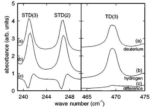
FIG. 3.  $1s \rightarrow 2p_{\pm}$  transitions of the two strongest STDs: STD(2) and STD(3) (left) and TD(3) (right) in the spectra of a pair of  $n$ -type phosphorus doped samples which had been heated (a) in a deuterium plasma for 34 h, and (b) in hydrogen plasma for 17 h. After normalizing the strengths of the absorption (increasing that from the deuterated sample), we obtained the difference spectra shown in (c), demonstrating the isotopic shift of the STD lines.
