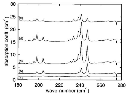
FIG. 1. The IR absorption spectra from STD centers in B-doped ( $2 \times 10^{14}$   $\text{cm}^{-3}$ ) samples annealed at 470 °C in a hydrogen plasma for (a) 5 h, (b) 10 h, (c) 20 h, (d) 40 h, and (e) 70 h. Spectra (a)–(e) are displaced progressively for clarity of presentation. Absorption lines usually ascribed to  $1s \rightarrow 3p_{\pm}$  transitions were very weak or absent.
