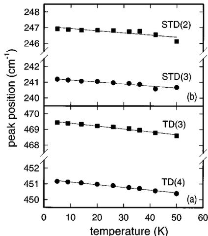
FIG. 2. The peak position of the absorption line corresponding to the transition  $1s \rightarrow 2p_{\pm}$  of (a) TD(3), TD(4), and (b) STD(2), STD(3), as a function of sample temperature in the range 5–50 K.
