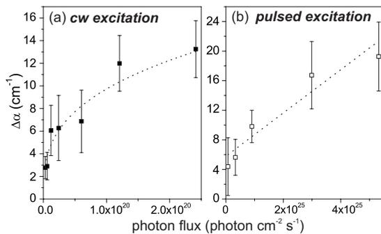
FIG. 5. Laser-induced absorption coefficient changes  $\Delta\alpha$  as function of the excitation photon flux  $\Phi$  for both (a) cw and (b) pulsed excitation ( $t_p=5$  ns) at 532 nm. The dashed lines represent fits by Eqs. (7) and (9), respectively.
