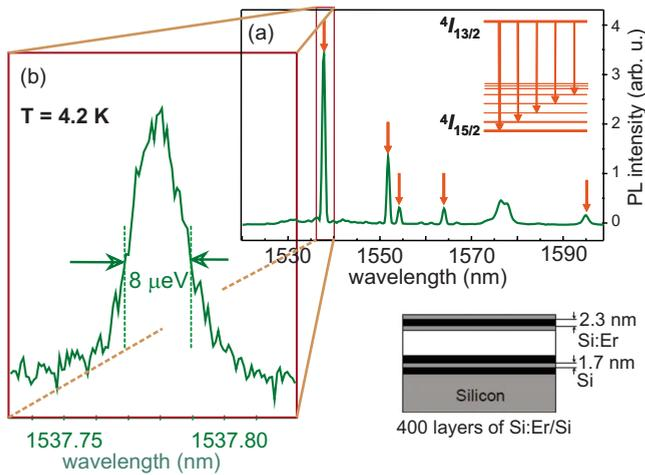
FIG. 2. (Color online) (a) PL spectrum of the Si/Si:Er multilayer structure, as measured at  $T=4.2$  K under cw excitation at 532 nm. (b) Detail of the studied Er-1 center related ultranarrow emission line at  $1.54 \mu\text{m}$ . Inset: sketch of the multilayer structure.
