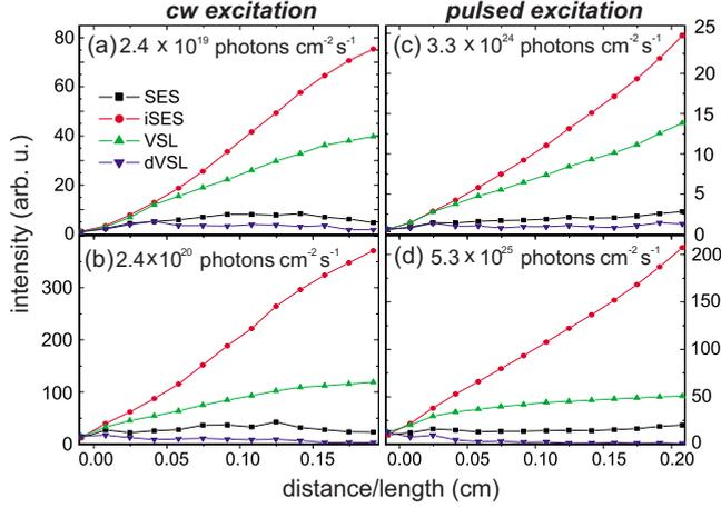
FIG. 4. (Color online) Comparison of the as-measured VSL and SES signals with the integrated SES and differential VSL signals, measured at  $1.54 \mu\text{m}$  Er-1-related emission for different excitation flux under [(a) and (b)] cw and [(c) and (d)] pulsed excitation at 532 nm. Measurements were done at low temperature  $T=4.2$  K.
