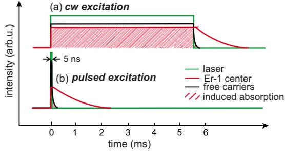
FIG. 6. (Color online) Sketch of the interplay between the free carriers and Er-1 luminescence lifetimes under laser illumination for (a) cw and (b) pulsed excitation ( $t_p=5$  ns). The striped areas represent the induced absorption at the emission wavelength of  $1.54 \mu\text{m}$  due to the free carrier absorption.
