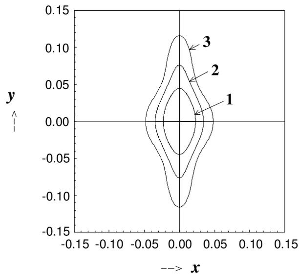
Fig. 2. Isointensity curves of a 1:1 mixture of oblate ( $q = 1$ ,  $\alpha = 56.9$ ) and prolate ( $q = 4.7$ ,  $\alpha = 48.5$ ) spheroids. The volumes of the particles are  $95 \text{ fl}$ . The isointensity curves 1, 2 and 3 represent intensities  $I(0)/2$ ,  $I(0)/4$ , and  $I(0)/10$  respectively ( $I(0)$  is the intensity at the center of the screen).
