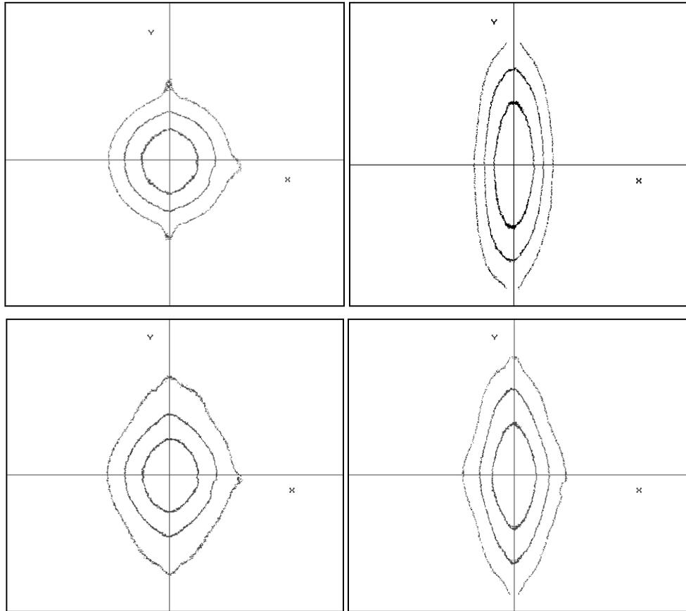
Fig. 3. Isointensity curves in the intensity patterns of suspensions with different fractions  $n_u$  of poorly deformable cells (top row: left  $n_u = 1.0$ , right  $n_u = 0.0$ ; bottom row: left  $n_u = 0.75$ , right  $n_u = 0.25$ ).
